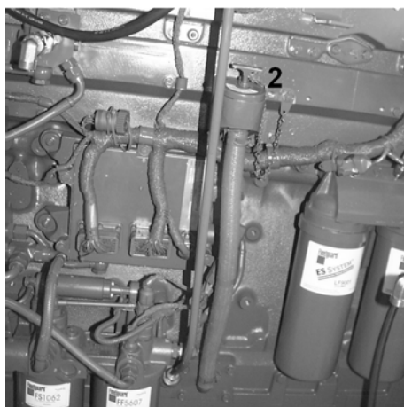
Fig. 5-10 Filler neck and dipstick
