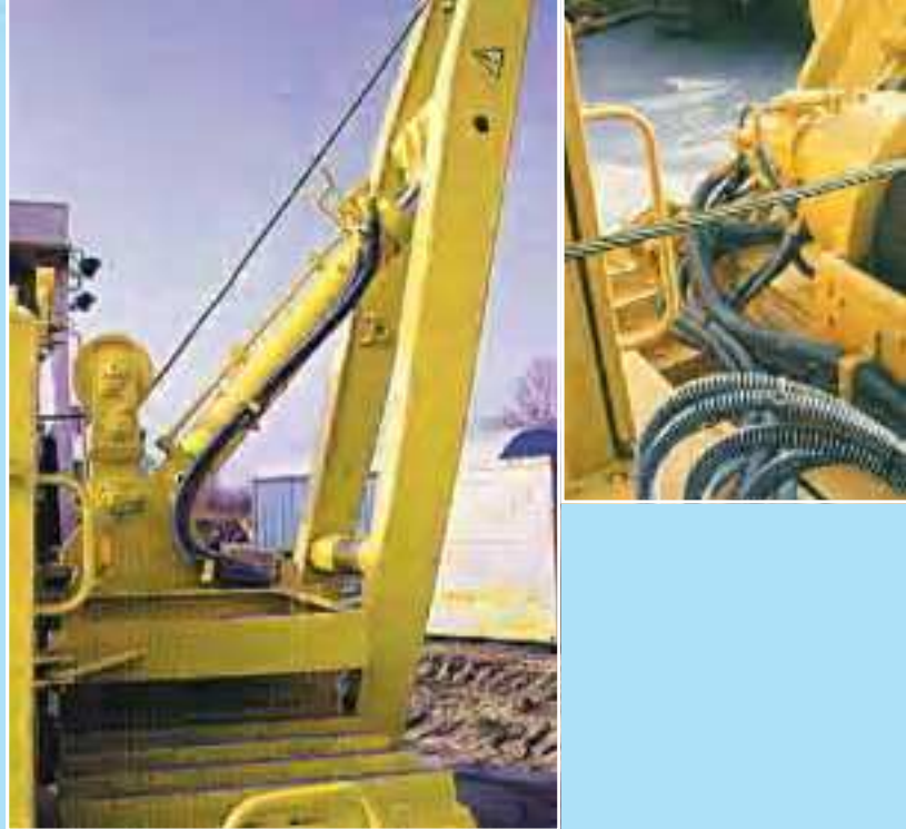
The boom can be adjusted precisely and without sudden jerks with a hydraulic cylinder.
