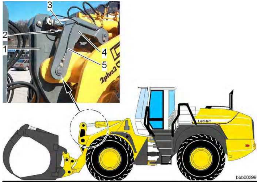
Tilt cylinder support
