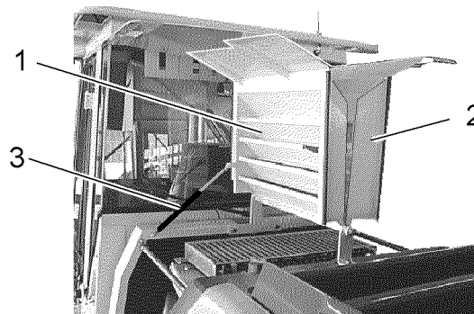
Cooling system hood
