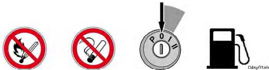
Safety while refuelling
