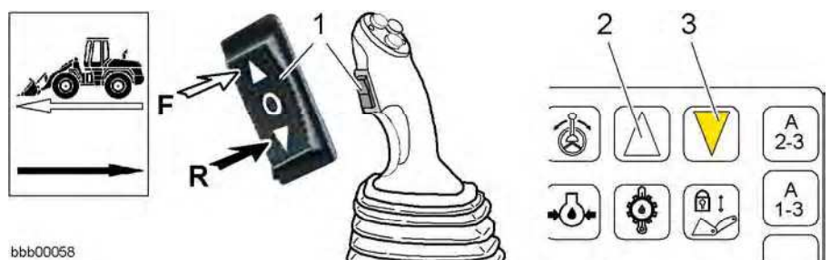
1 Travel direction switch 3 Reverse travel direction symbol field 2 Forward travel direction symbol field
