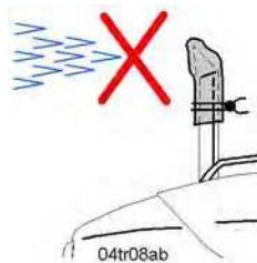
Blocking off the exhaust pipe opening
