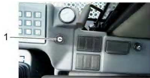
Ignition switch position
