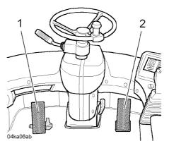
Brake / inching pedal – gas pedal
