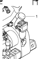
Pour the fresh oil in through filler neck 1 up to the marking MAX on the oil dipstick.
