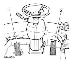
Brake- inching pedal and gas pedal
