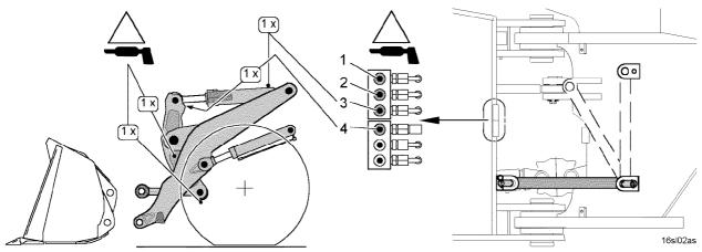
Lubrication points on the left-hand side of the central lubrication rail
