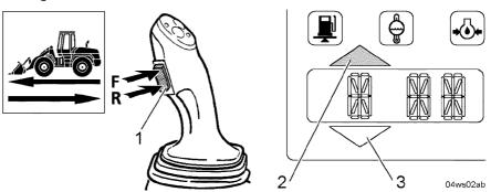
Switch for travel direction and display unit
