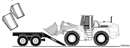
Loading the vehicle onto the transporter
