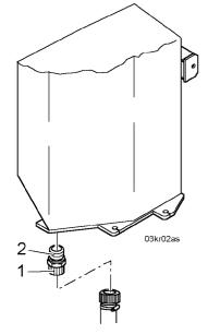
Draining off condensate from the fuel fine filter
