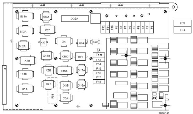
Control circuit board A12 with plug-in fuses F1-18
