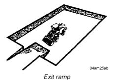
• To make an exit for the vehicle: dig out the centre of the ramp.
