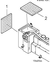
Modification The existing fresh air filter has been replaced with a foam pre-filter and a foam fine filter.
