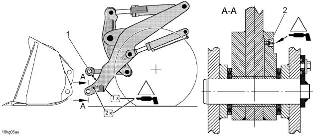
Lubrication points - bucket coupling
