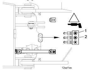
Lubrication points on the right-hand side of the central lubrication rail
