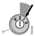
• Switch on the electrical system by turning the starting key to position - I -.
