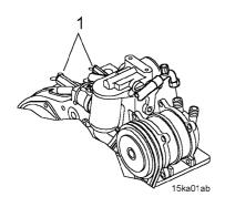
The shut-off valves 1 on the thermostat housing of the diesel engine must be open so that the cab can be heated.
