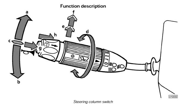
Functions of the steering column switch when activated in direction:
