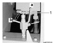
Deactivate the hydraulic quick-change device with the changeover valve (block).
