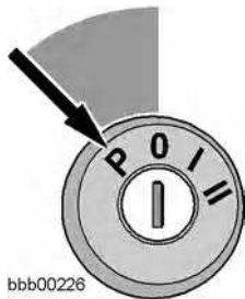
Ignition switch parking position
