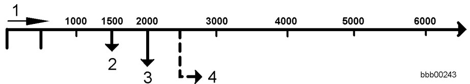
Oil change intervals according to sample analysis and laboratory report
