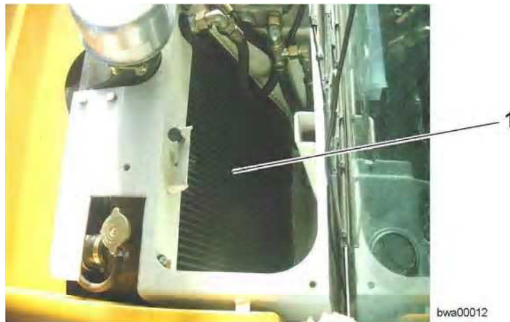
Cleaning the cooler units
