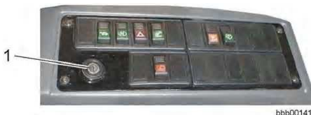
Ignition switch position
