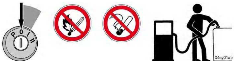
Safety while refuelling
