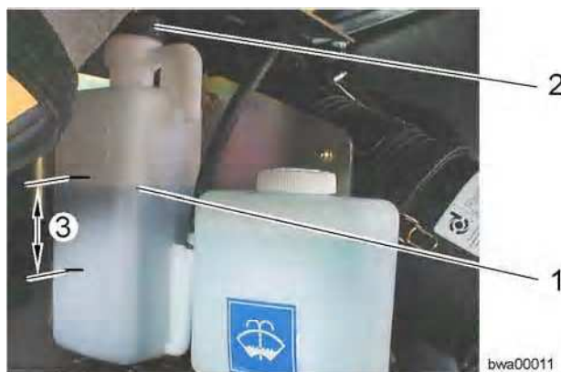
Checking the coolant level
