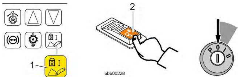
Working hydraulics lockout
