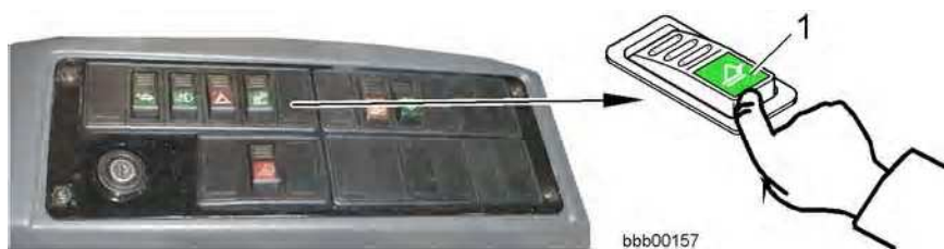
Switches on the side console
