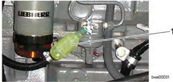
Replacing the fuel pre-filter
