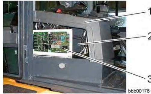
Fuse box with A4 control board
