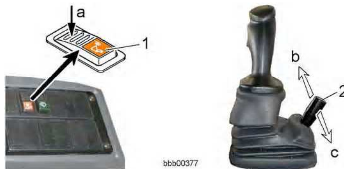
Reducing the operating pressure
