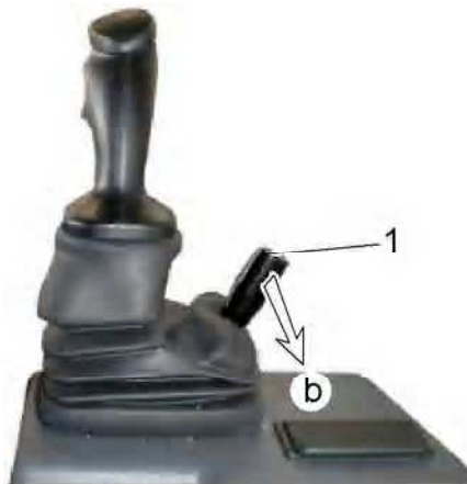
Unlocking the quick-change device
