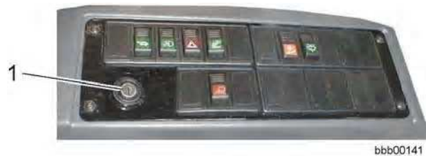
Ignition switch position
