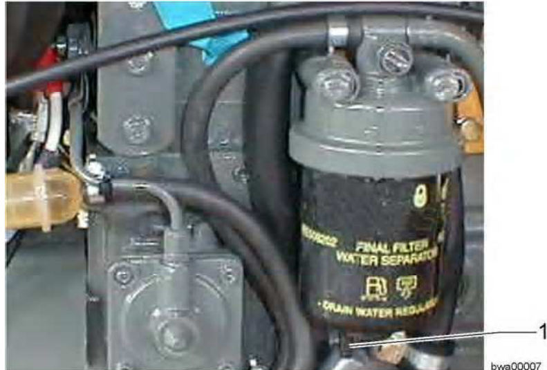
Draining off condensate
