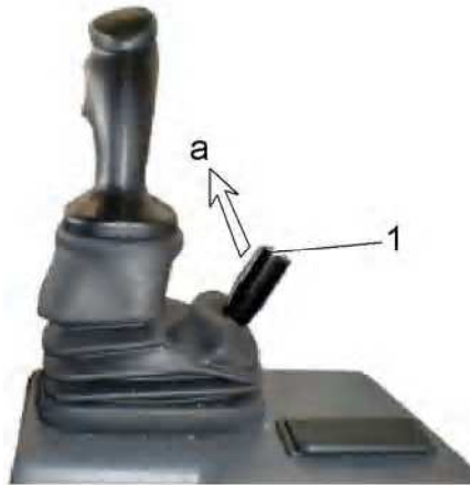
Locking the working attachment
