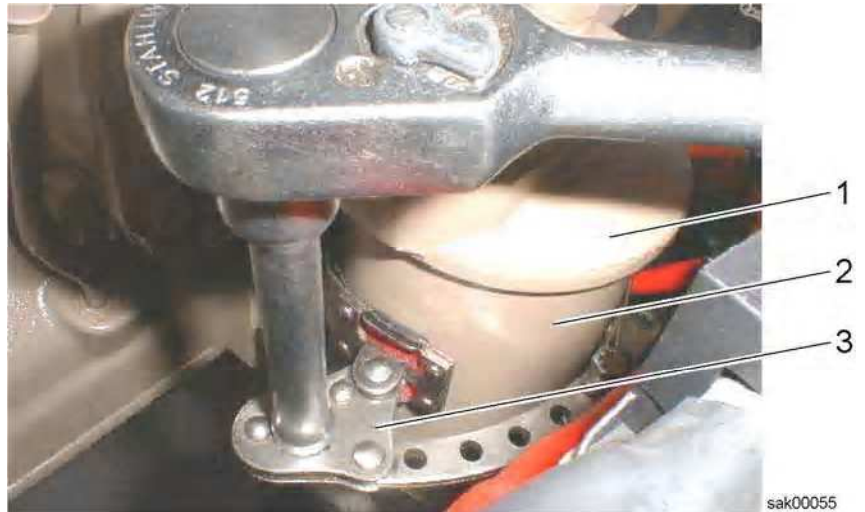
Unscrewing the oil filter
