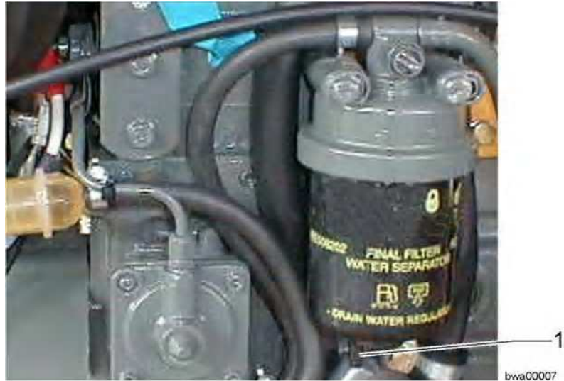
Draining off condensate
