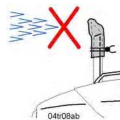
Blocking off the exhaust pipe opening
