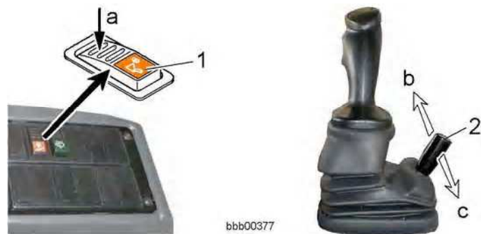
Reducing the operating pressure
