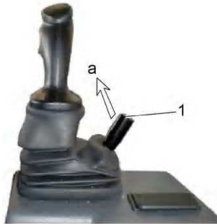
Locking the working attachment
