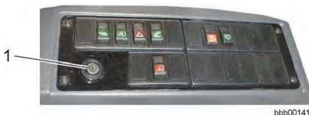
Ignition switch position
