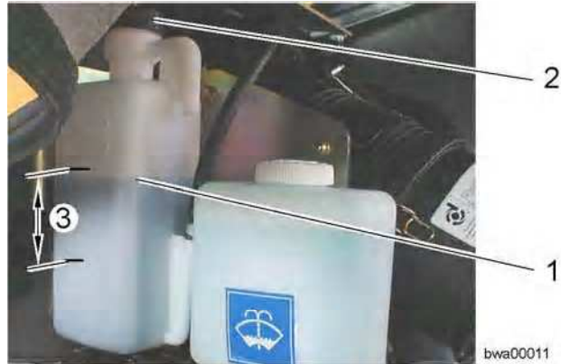
Checking the coolant level
