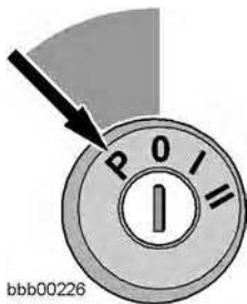
Ignition switch parking position
