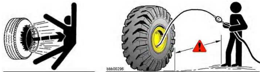
Checking and adjusting the tyre pressure
