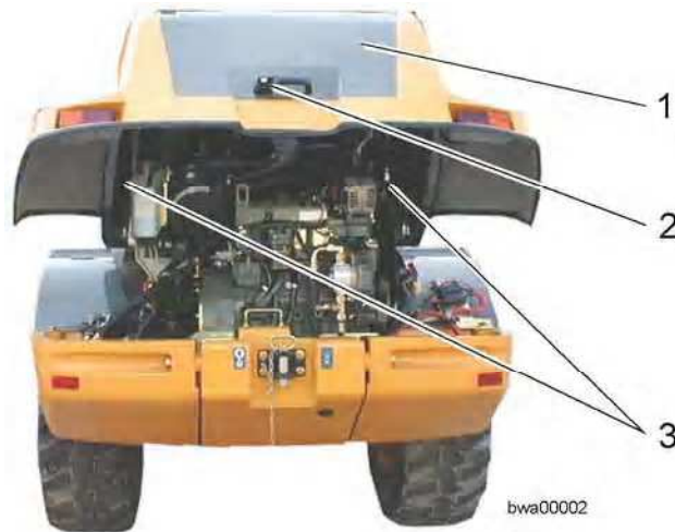
Engine compartment hood
