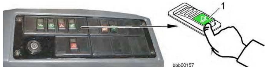
Switches on the side console
