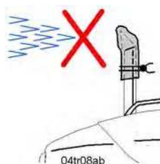
Blocking off the exhaust pipe opening
