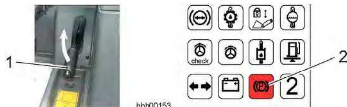
Display unit and parking brake switch
