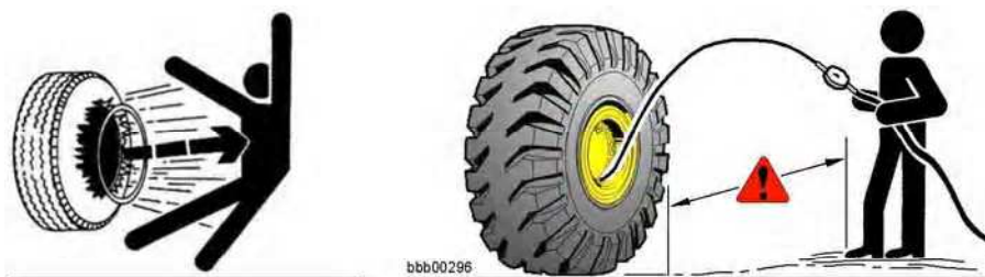
Checking and adjusting the tyre pressure
