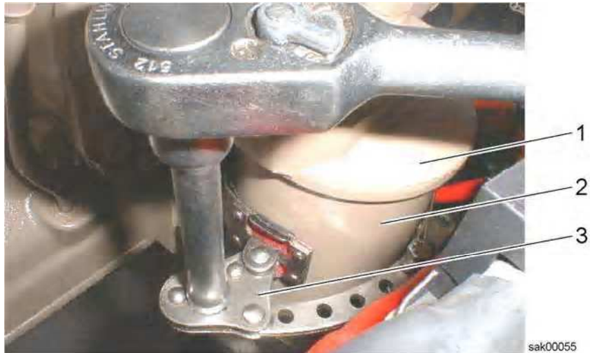
Unscrewing the oil filter
