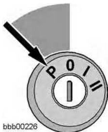
Ignition switch parking position
