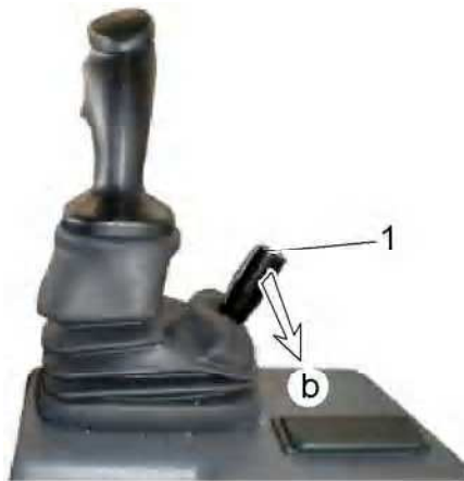
Unlocking the quick-change device
