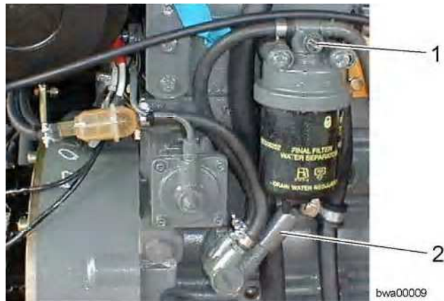
Bleeding the fuel system
