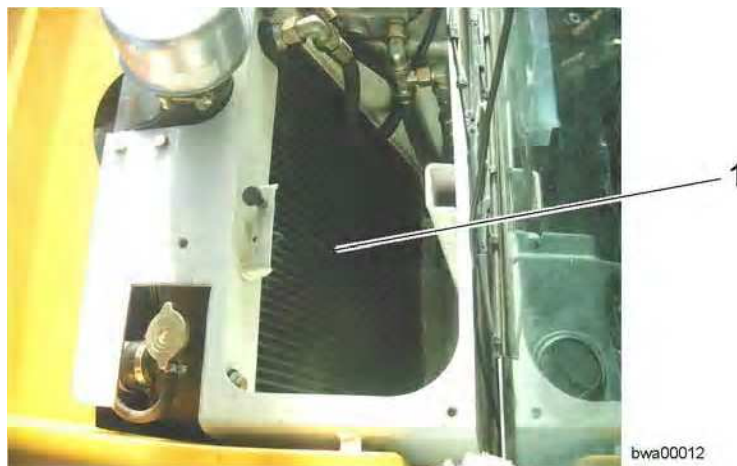
Cleaning the cooler units
