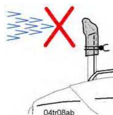
Blocking off the exhaust pipe opening
