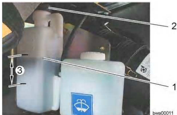
Checking the coolant level
