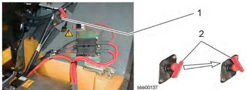
Battery main switch
