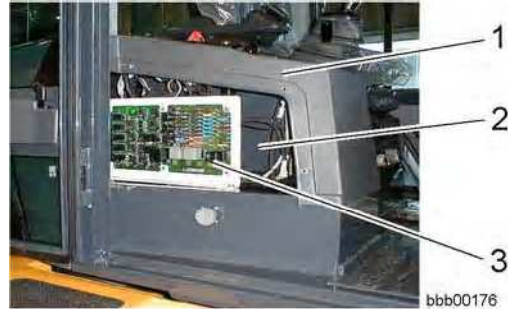
Fuse box with A4 control board
