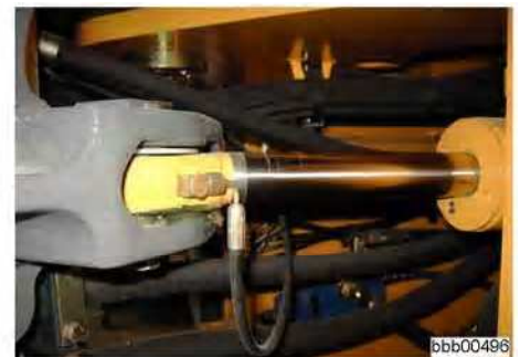
Steering cylinder lubrication points
