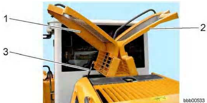
Cooling system hood
