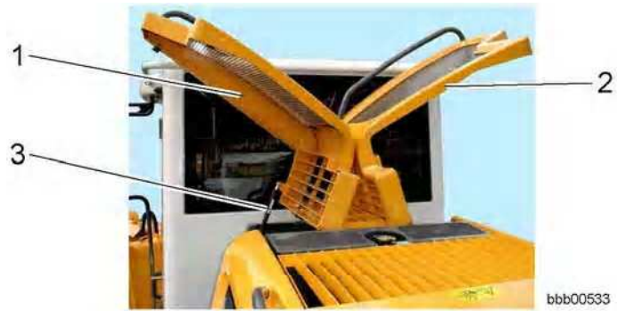
Cooling system hood
