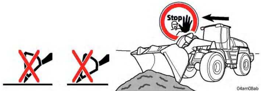
Impermissible bucket positions
