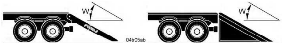
04tr05ab Ramp inclination
