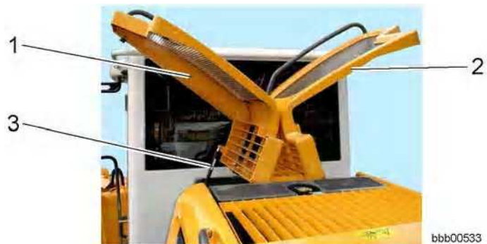
Cooling system hood
