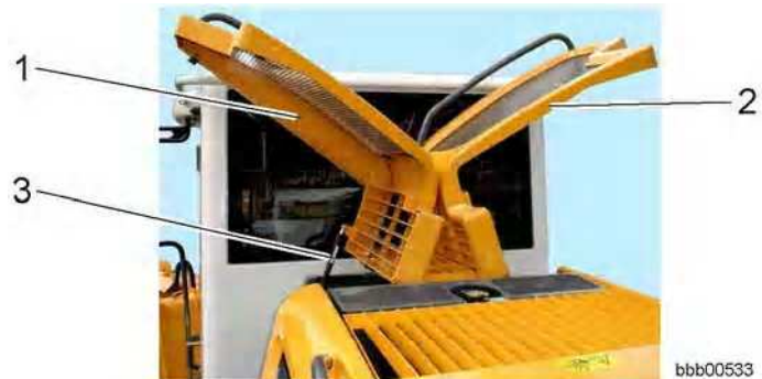
Cooling system hood
