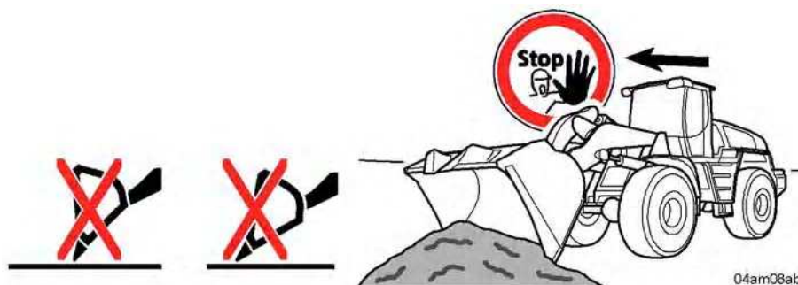
Impermissible bucket positions
