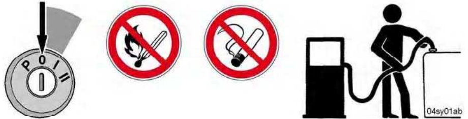
Safety while refuelling
