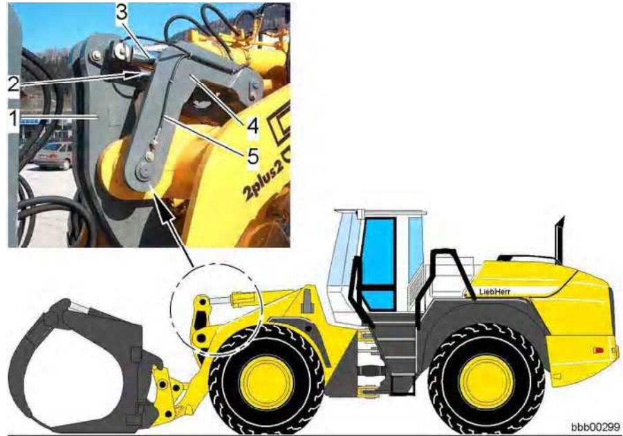
Tilt cylinder support
