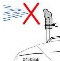
Blocking off the exhaust pipe opening
