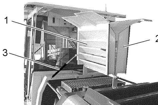
cooling system hood
