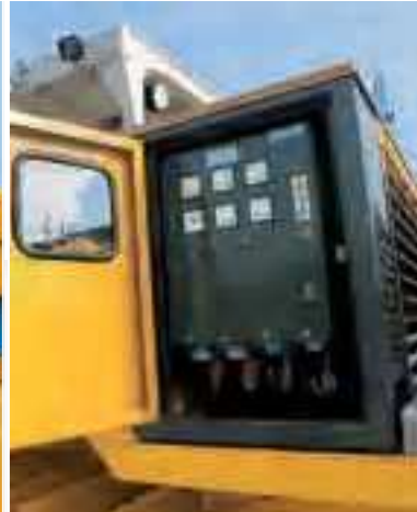
The electric generator is driven hydraulically for constant weld quality.
