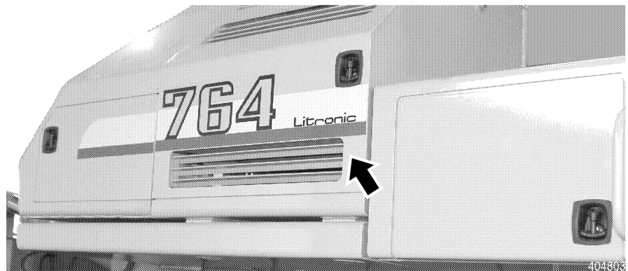
Reservoir - oil cooler
