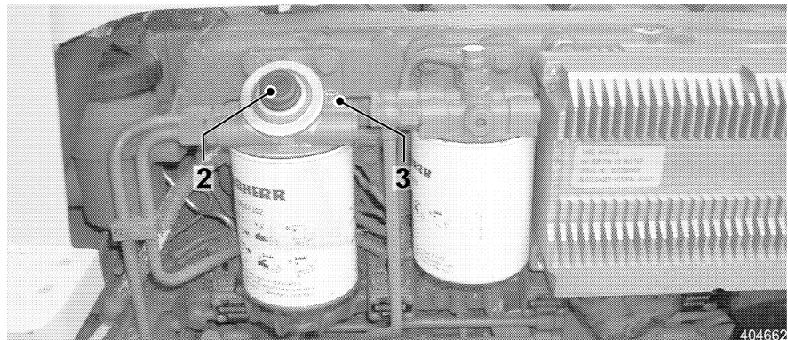
Breather screw on the filter head of the fuel prefilter
