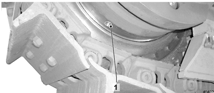
Drain plug – slip ring area
