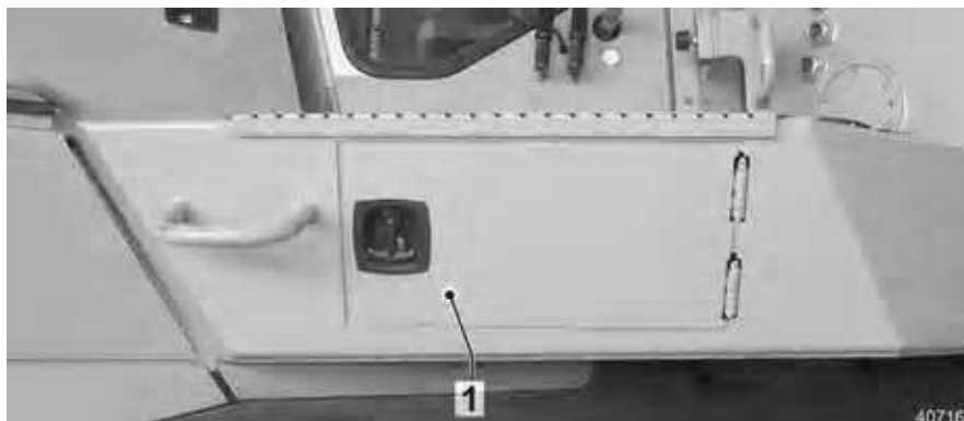
Access – refueling pump
