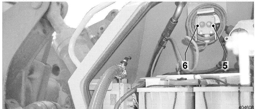
Switch – Refueling pump
