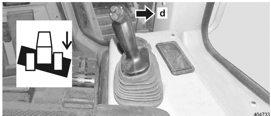
Tilt the dozer blade to the right
