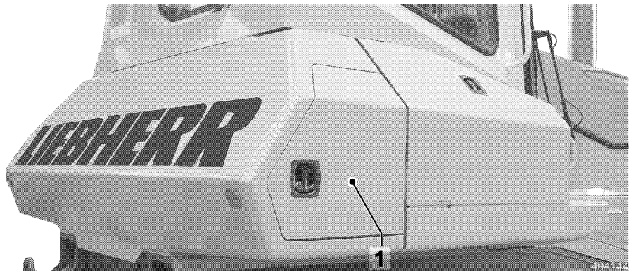
Access – Refueling pump
