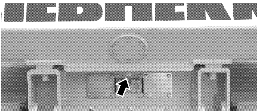
Shut off valve - fuel tank
