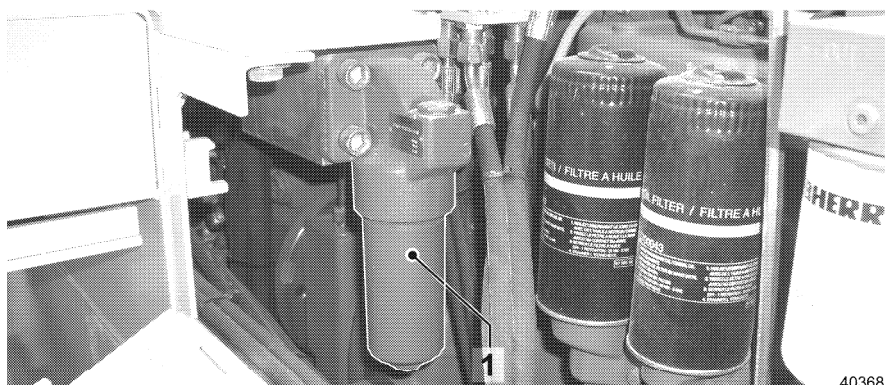
Filter - replenishing circuit
