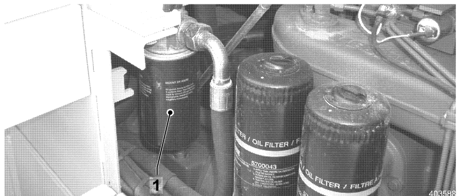
Filter - replenishing circuit
