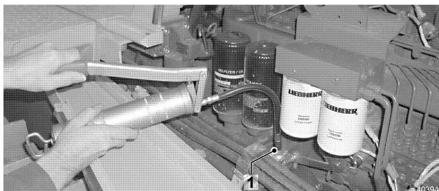
Lube point - oscillating axle bearing
