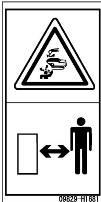
(16) Prohibition of unauthorized entry into Off-Limit working area (09829-H1681)
