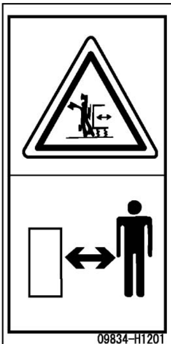
(19) Precautions for access to the grizzly while in operation (09834-H1201)
