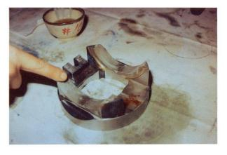
5. Rub both sliding surfaces with paper to remove both the oil and the lapping powder.
