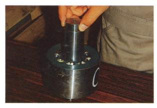
Push down on the valve plate with a force of 4 - 5 kg, and move the valve plate backwards and forwards 90° two or three times.
