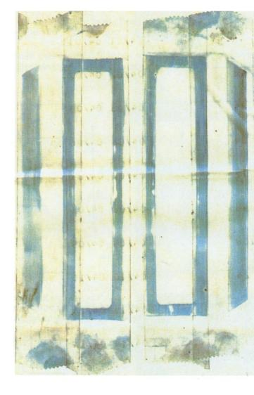
2. Contact between end cover and valve plate on KMV Series
