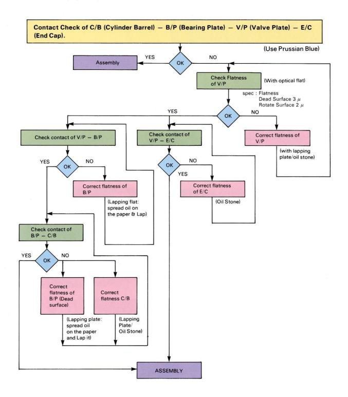
This example is shown how to correct and check the flatnesses of the vital parts surfaces of piston pumps and motors.
