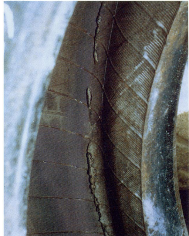
8. Cord drag on inner face of tire
