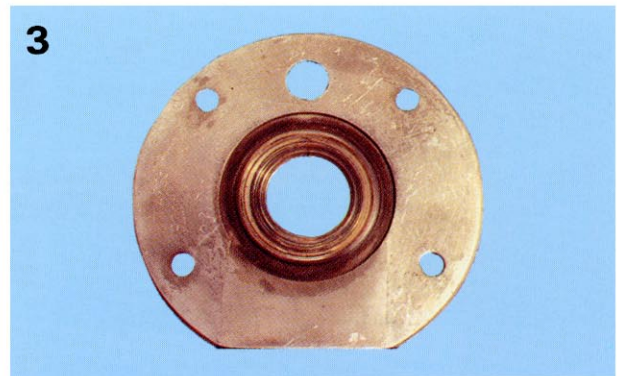
Thrust bearing excessively worn or scuffed due to the lack of lubricating oil.
