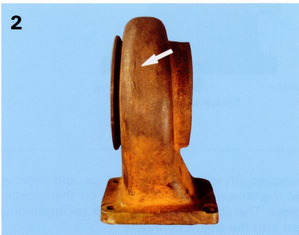
Turbine housing with heat cracks.
