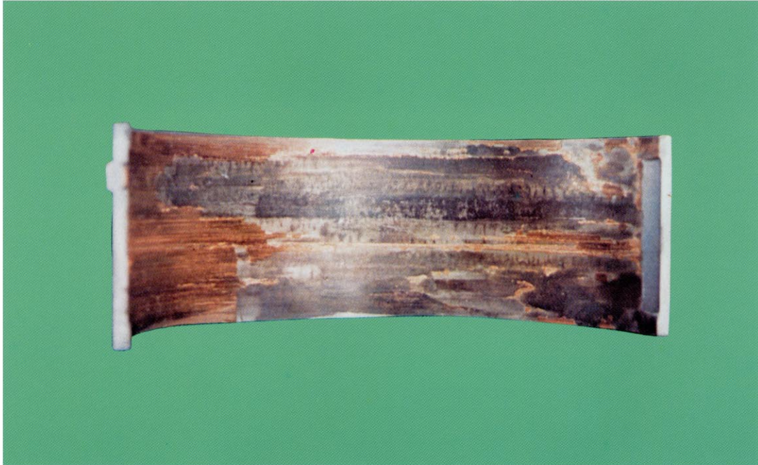
Phenomenon: Both surface in bearing and shaft are melted and catastrophic aspect is discernible. This photograph indicates the damage example resulted from decrease of viscosity in oil.
