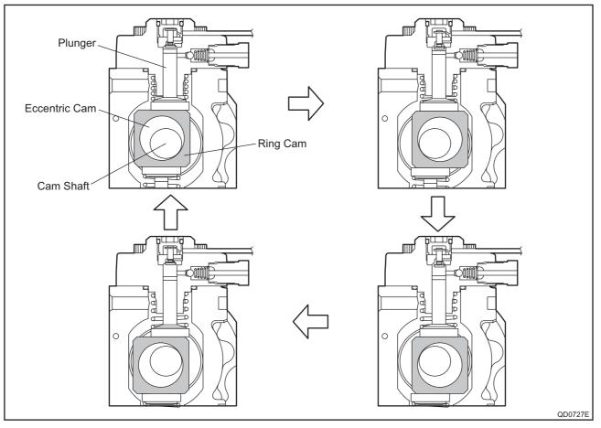
c. The plunger and the suction valve are attached to the ring cam. The feed pump is connected to the rear of the cam shaft.
