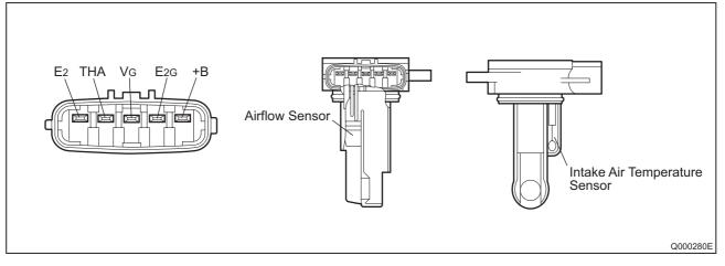
c. The airflow sensor is installed to the rear of the air cleaner, and consists of a heater, thermometer, intake air temperature sensor, and control circuit (base). It diverts a portion of the intake air from the air cleaner and measures the intake airflow at the hot-wire measuring part.
