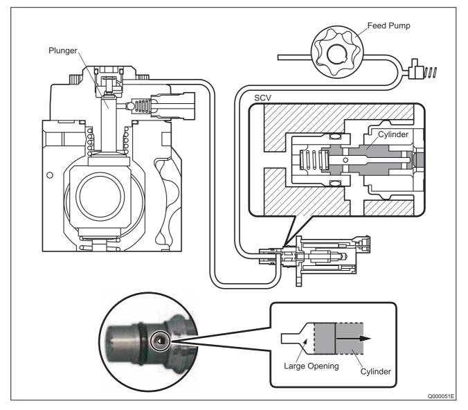
Short time ON duty  $\rightarrow$  large valve opening  $\rightarrow$  maximum intake quantity
