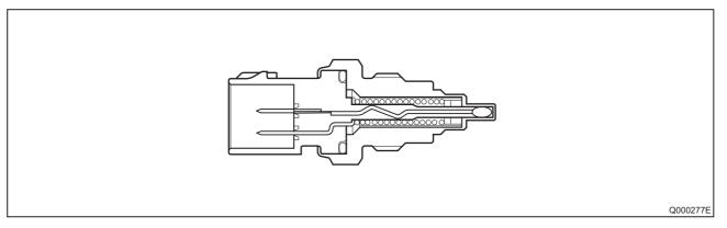
b. The sensor uses a thermistor, which varies resistance according to temperature. As the ECU applies voltage to the thermistor, it uses a voltage resulting from the division of the computer internal resistance and the thermistor resistance to detect the temperature.
