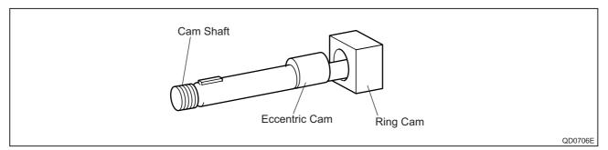
b. As the cam shaft rotates, the eccentric cam rotates eccentrically, and the ring cam moves up and down while rotating.
