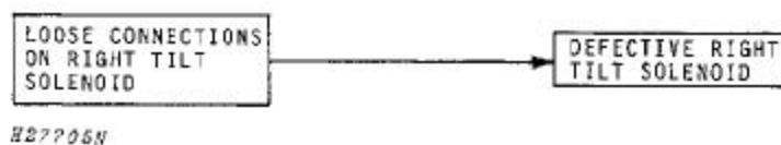
Fig. 11-Combine will not Level Manually or Automatically to the Right
