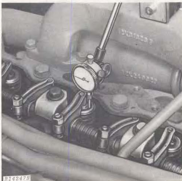
Fig. 6-Checking Valve Lift (6-Cylinder shown)
