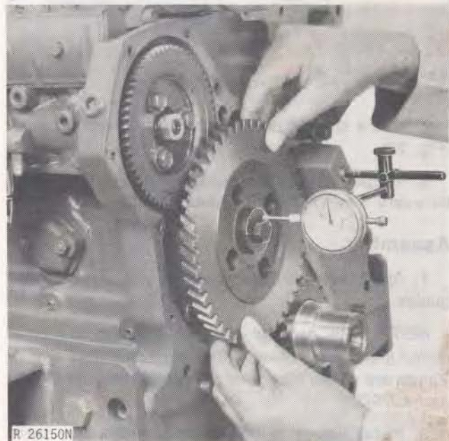
Fig. 25-Checking Camshaft End Play
