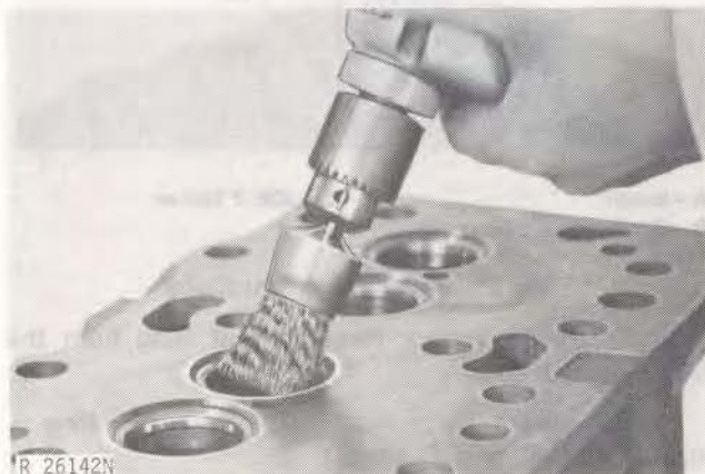
Fig. 16—Cleaning Valve Seats
