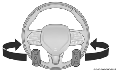
Remote Sound System Controls
