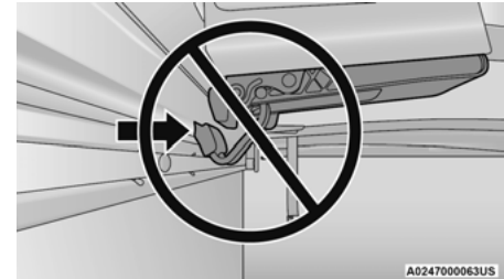
Improper Clamp Position
