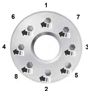
8-lug nut torque sequence.
