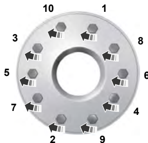
10-lug nut torque sequence.
