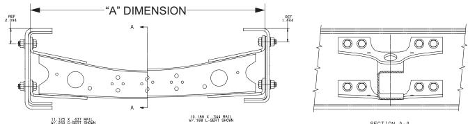
572-057 INVERTED MOUNTED REAR CLOSING CROSSMEMBER 572-065 INVERTED MOUNTED REAR CLOSING CROSSMEMBER AFT 82 INCHES FROM REAR SUSPENSION CENTERLINE
