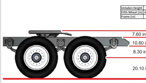
**Frame Height** =  $\frac{1}{2}$  the tire diameter + Rear Suspension Ride Height + Frame Height.
