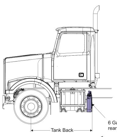
6 Gal DEF tanks mount rear of Fuel tanks
