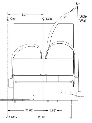
Typical seat belt installation for 2-man, box base seat
