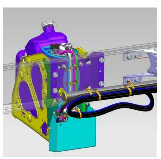
The truck comes equipped with max length DEF lines and harness to accommodate easy repositioning of DEF Tank
