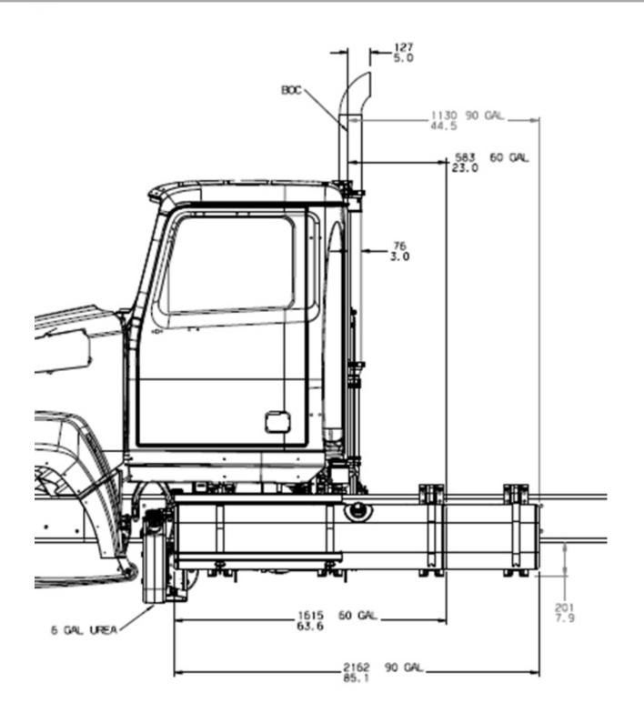
Note: Rectangular fuel tanks are not available on 4700SB with a DD 13 engine for Snow Plow configurations.
