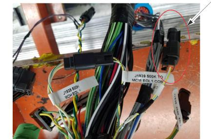
J1939 End of Line (EOL) Connections (Image referencing Cummins EOL)
