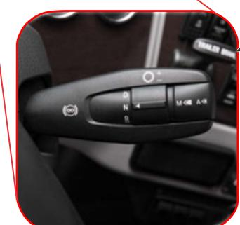
4700 Enhanced Gear selection, engine brake and manual shifting
