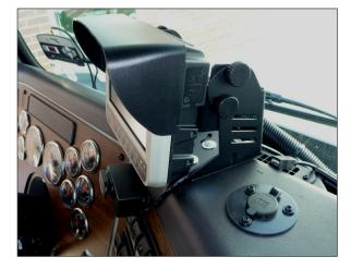
**AWTI Camera Mounted using** common mounting pattern
