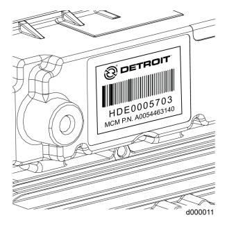
Figure 26. Motor Control Module Label
