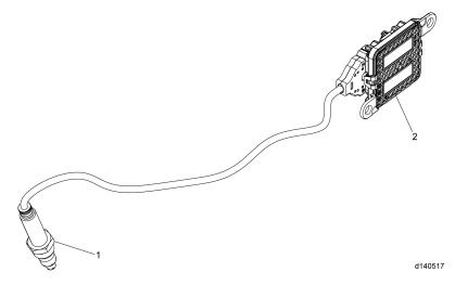
1. Soot Probe 2. Sensor Control Unit (SCU) Figure 32. Soot Probe and Sensor Control Unit (SCU)
