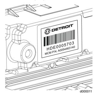
Figure 22. Motor Control Module Label
