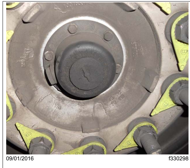
Fig. 9, Normal Oil Venting
