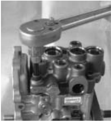
Remove the hydraulic head CMP fixing bolt.
