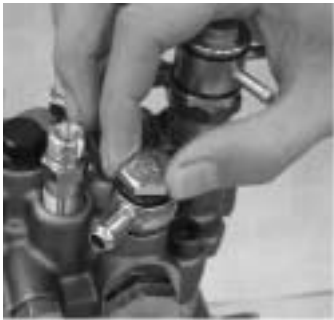
Install the joint, (FO inlet).
