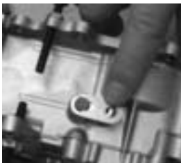
Remove the removal stop, (governor lever shaft).
