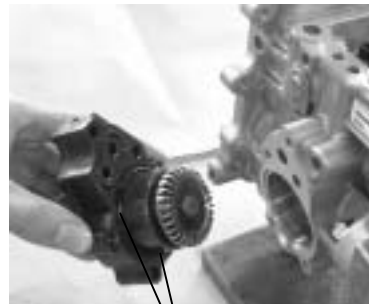
Do not loosen two bolts (A)
