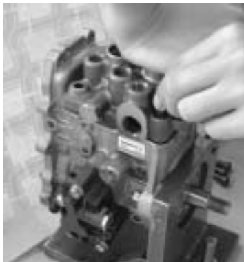
Install the hydraulic head CMP.
