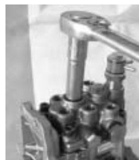
Remove the delivery valve and gasket. Remove gasket
