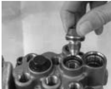
Install the plug with new copper packing, (barrel).
