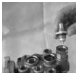
Remove the thermo element.
