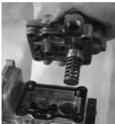
Remove the hydraulic head CMP.
