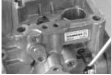
Remove the whirl-stop, (tappet).
