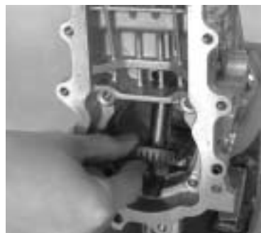
Remove the transmission shaft CMP.
