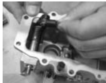
Remove the spring.
