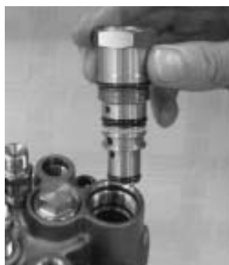
Install the holder with new O-ring, (timer).
