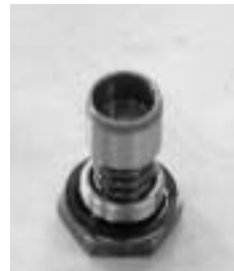
Remove the plug, (accumulator). Make sure that the seal washer remains on the plug.
