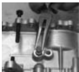
Pull out the governor lever shaft.
