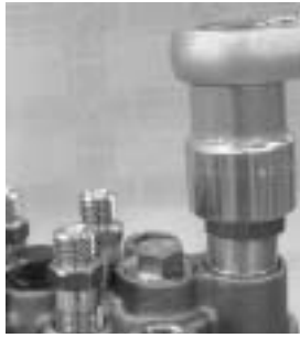
Fasten the thermo-element.
