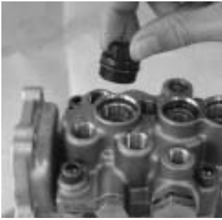
Install the plug, (distribution shaft).
