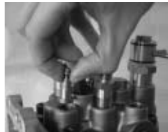
Remove the delivery valve and gasket.
