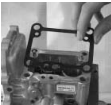
Remove the packing.
