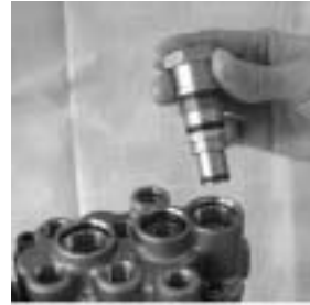
Remove the holder and gasket, (timer)
