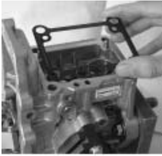
Install the hydraulic head CMP.
