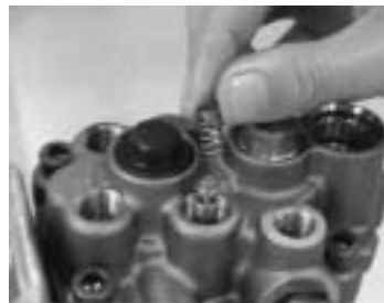
Install the spring, (delivery).
