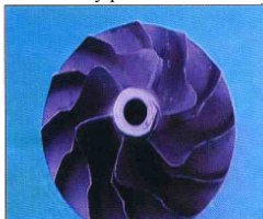
Compressor impeller damaged by dust
