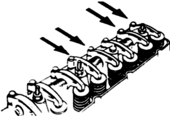
Top dead center of the fourth cylinder compression stroke
