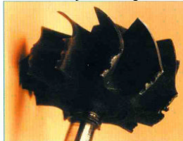
Turbine impeller damaged by particles
