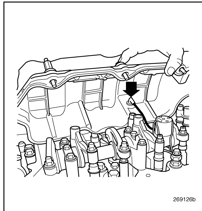
Figure 163 — PowerLeash™ Internal Control Wire Removal
