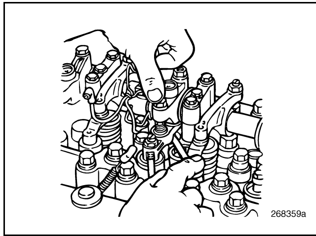
Figure 567 — Checking Valve Yoke Adjustment
