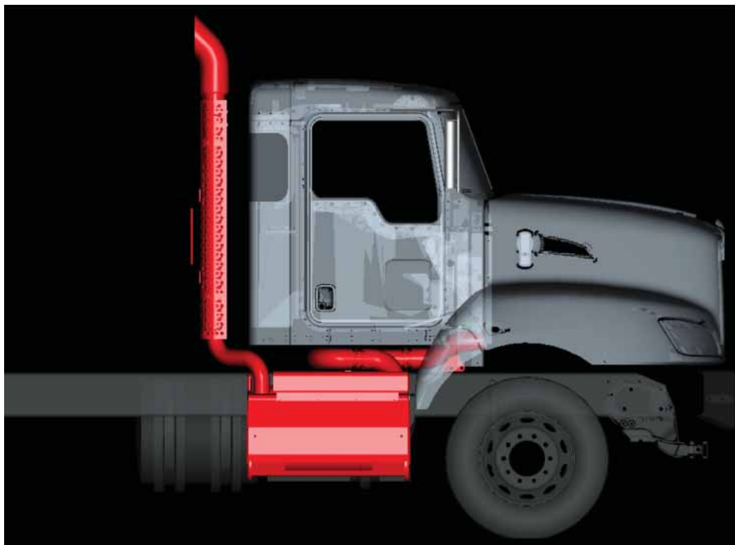
FIGURE 4-16: Right view of Right Hand Under DPF and SCR with Single Back of Cab Tailpipe
