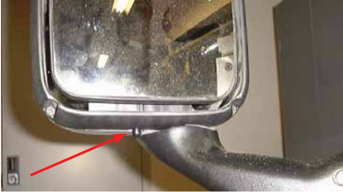
FIGURE 2-4: Aerodynamic Mirror OAT Sensor Location
