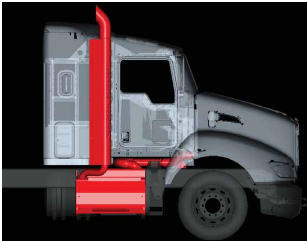
FIGURE 4-24: Right View of Right Hand Under DPF and SCR on Aerocab with Single SOC Tailpipe
