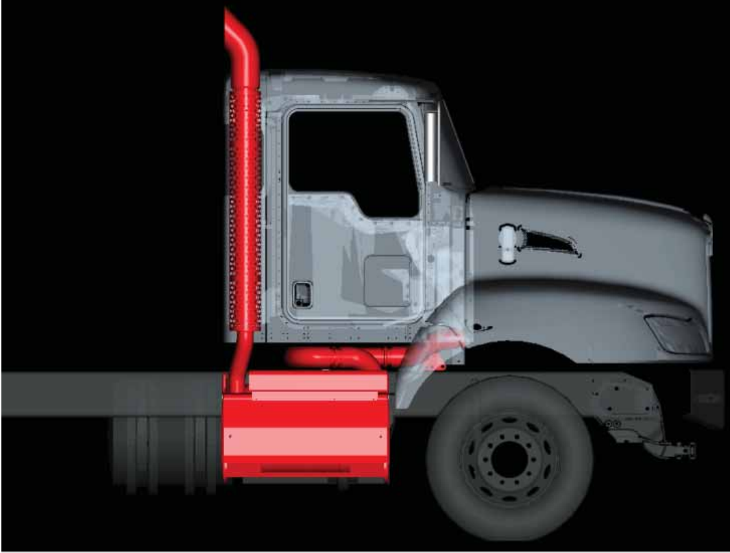
FIGURE 4-12: Right View of Right Hand Under DPF and SCR with Single SOC Tailpipe
