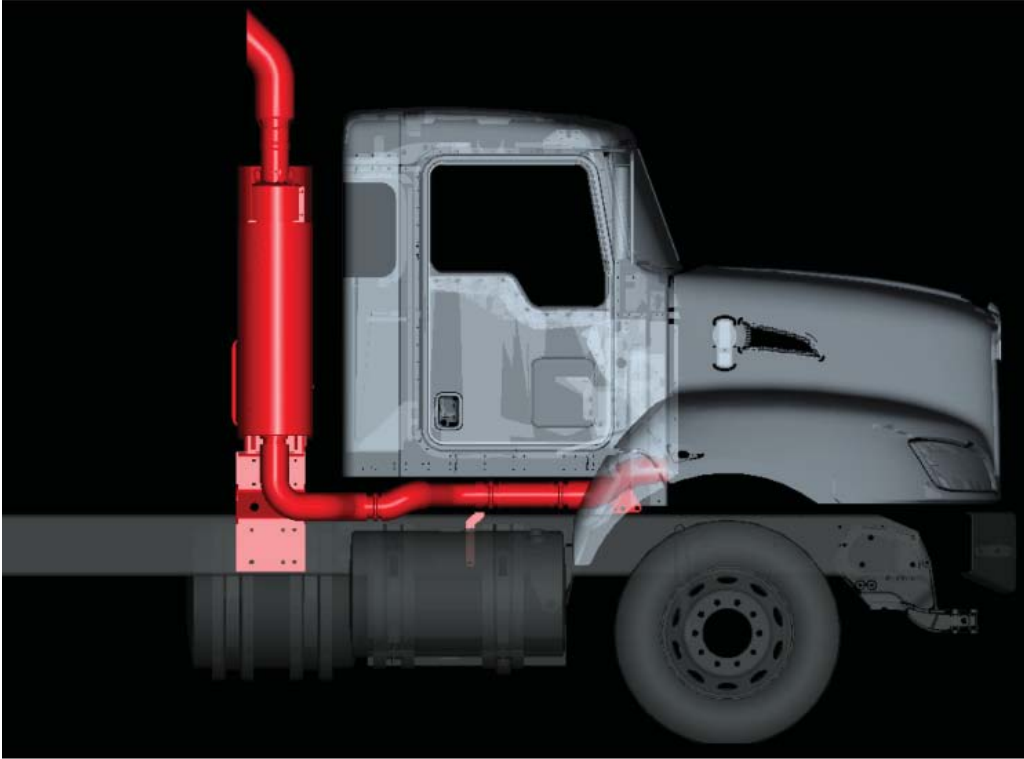
FIGURE 4-20: Right View of Vertical DPF and SCR
