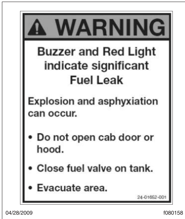
Fig. 19.5, Exterior Warning Sticker
