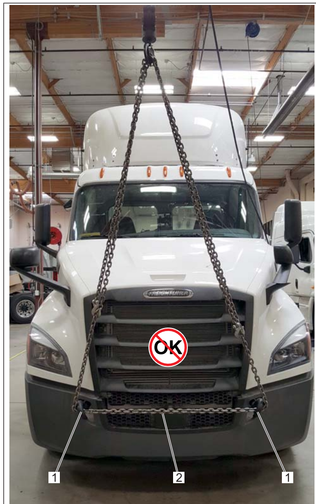
Fig. 24.12, Moving the Stinger and Crossbar Under the Bumper
