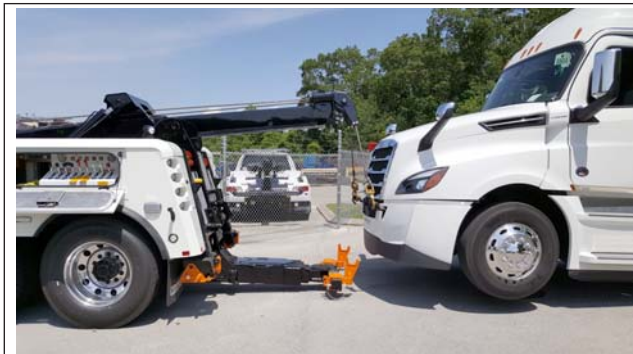
Fig. 24.14, Backing the Tow Truck with Lift Adaptors on the Crossbar
