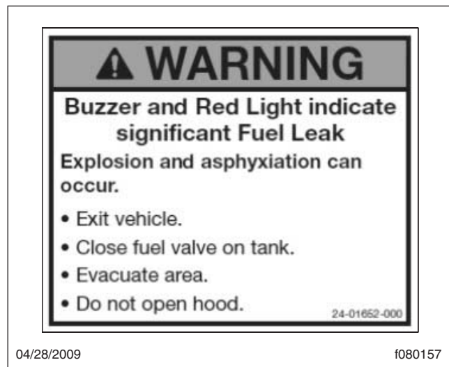
Fig. 19.4, Interior Warning Sticker
