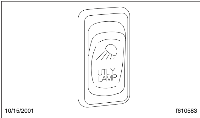
Fig. 5.10, Utility Light Switch
