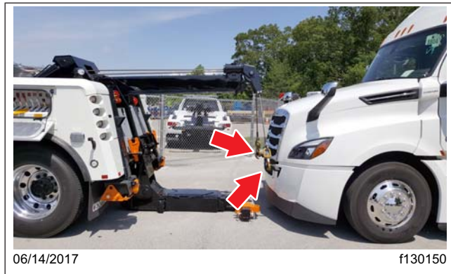
Fig. 24.11, Tow Cables Connected to the Tow Hooks
