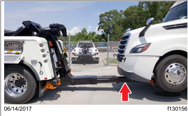
Fig. 24.17, Retracting the Recovery Boom
