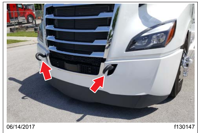
Fig. 24.8, Tow Hooks Installed, Facing Down
