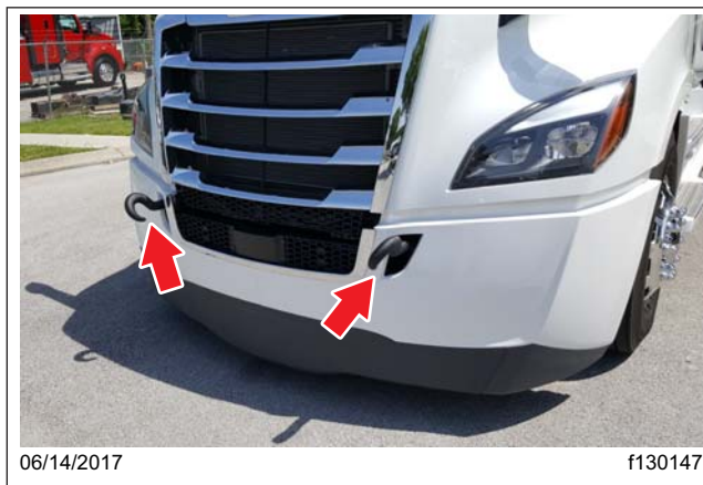
Fig. 23.4, Tow Hooks Installed, Facing Down
