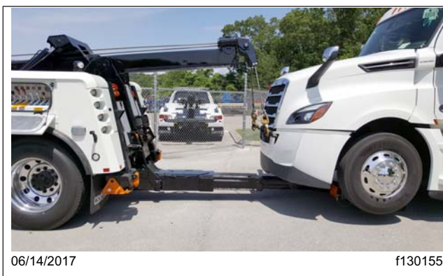
Fig. 23.12, Stinger with Lift Adaptors Under the Axle (tow truck shown)
