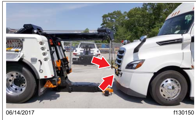
Fig. 23.7, Tow Cables Connected to the Tow Hooks
