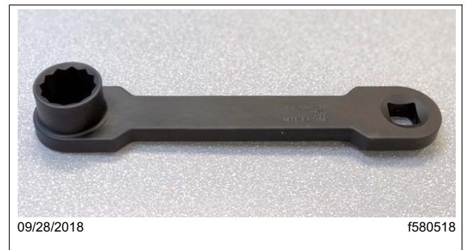
Fig. 5, DDC DSNCHA018005 30mm Air Disc Brake Caliper Brake Bolt Torque Adaptor
