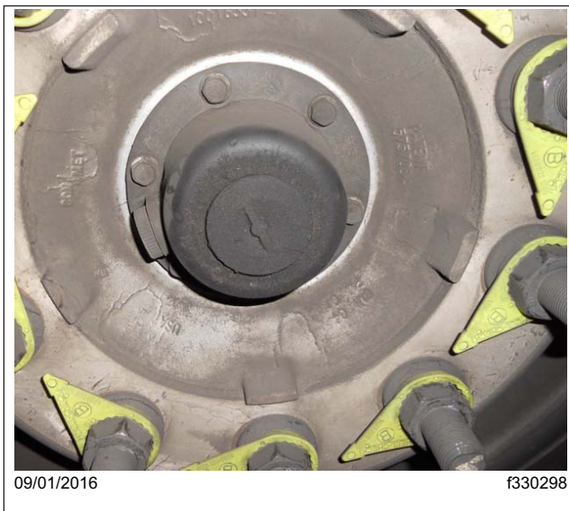
Fig. 13, Normal Oil Venting
